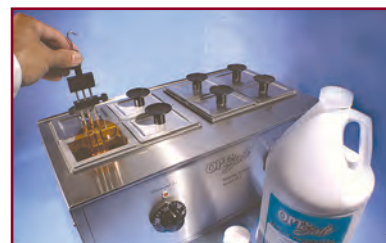
Tinting is simply done by dipping lenses into hot dye solution.
